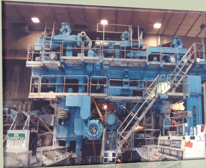
PC-590 was applied to the Press Section on the wet end of a paper machine while the surface was still damp.
